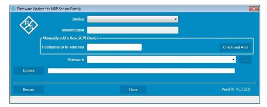
The program automatically starts scanning for R&S NRP-Zxx power sensors. When the scan is completed, all recognized power sensors are listed in the "Device" dropdown control.
