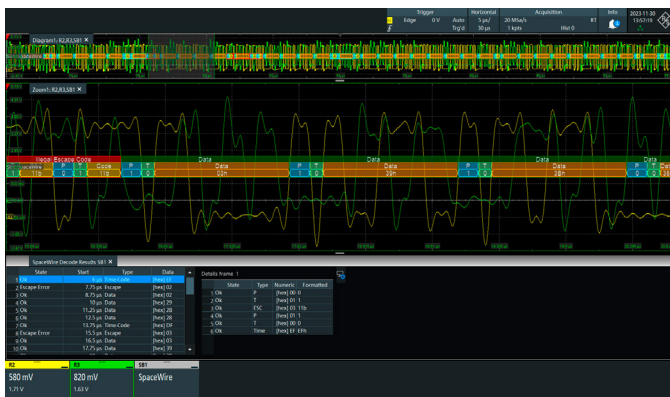
SpaceWire (left side) and MIL-STD-1553 (right side) decode on the R&S®RTO6 oscilloscope showing data and control characters, control codes and error messages of a continuous data stream.
