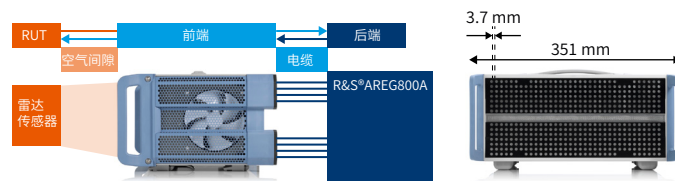
图9: 传感器布置和R&S®QAT100尺寸
