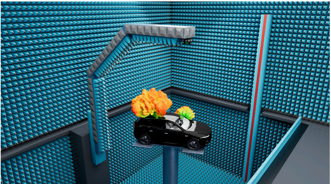
Fully anechoic OTA antenna test chamber for testing and verifying antenna modules integrated into a vehicle
