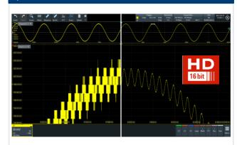
The low-noise frontend and 10 GHz single-core A/D converter are the foundation for the extraordinarily high measurement accuracy and dynamic range of the R&S\*RTO6 oscilloscopes. The HD mode activates a configurable hardware lowpass filter, increasing the vertical resolution to up to 16 bit and 9.4 ENOB. Since filtering reduces quantizing noise, signal details become visible.
