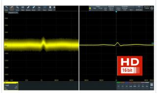
The unique digital trigger system from Rohde & Schwarz uses the sampling points of the A/D converter in the acquisition path so the trigger system's input data is identical to the displayed signal. The trigger system runs in high definition (HD) mode with up to 16-bit vertical resolution. This results in very high trigger sensitivity. You can reliably isolate even the smallest signal details.
