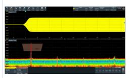
The R&S®RT06 provides multichannel FFTs that enable spectrum analysis on every channel with individual settings (center frequency, frequency span, resolution bandwidth) and an update rate of > 1 000 000 waveforms/s. The overlapping FFT and zone trigger in the frequency domain help to detect and analyze challenging EMI problems such as sporadic emissions.
