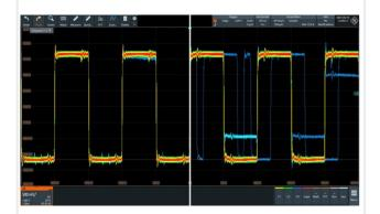
R&S®RT06 oscilloscopes display up to 1 million waveforms/s.
