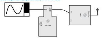
6. Press the power button once to turn on ESCU. When turned on, the power LED on ESCU will light up in green and status LED on ESCU-Z01 will turn from amber to green
