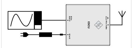
2. Connect a relevant signal source (e.g., transducer) to 'RF In' on ESCU
