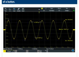
QuickMeas: automatic measurement and graphical display at the push
