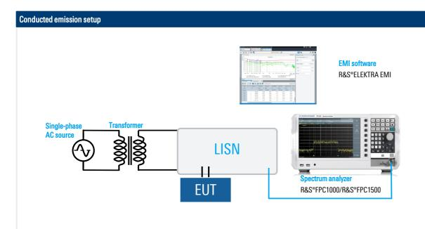
For line-conducted interferences measurement. The setup analyzes the level of RF energy coupled from the EUT to the mains supply.
