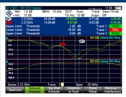
For cable loss and antenna testing and characterization as well as distance to fault measurements. Two-port capability for transmission measurements
