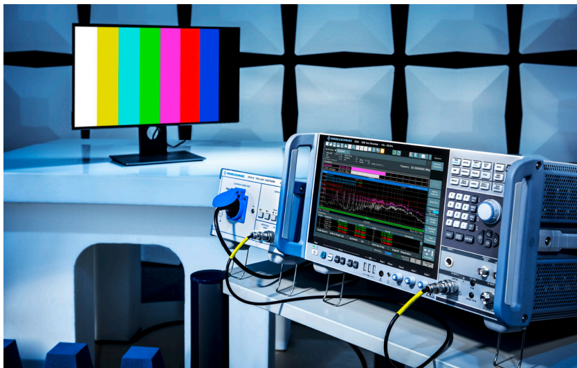
The powerful R&S®ESW forms the core of an EMI compliance test system.
