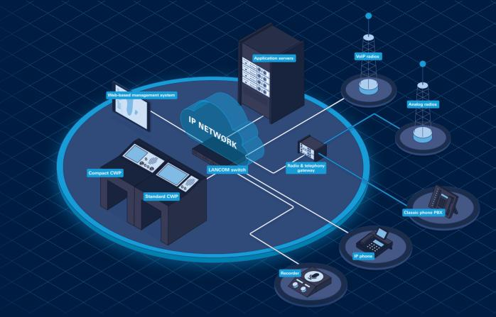
CERTIUM VCS consists of intelligent controller working positions (CWP) and redundant application servers. CWPs communicate directly to radios and telephones via VoIP. Application servers flexibly enhance the solution with additional features such as conference calls, session replication, radio control, best-signal selection, role handing and others.
