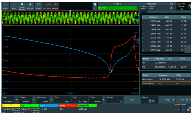
Frequency response analysis with the MXO 4 series
