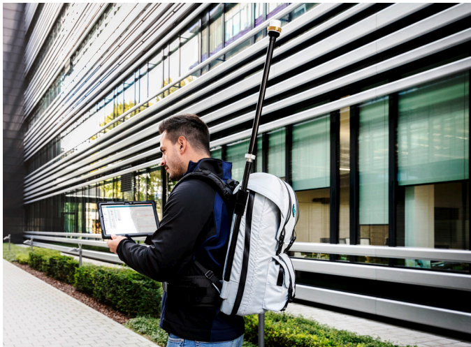
Walk testing with the R&S®FR4 Freerider 4 backpack system using the R&S®TSMS-OMN70 antenna mounted on the R&S®FR4-5G-A3 antenna holder.
