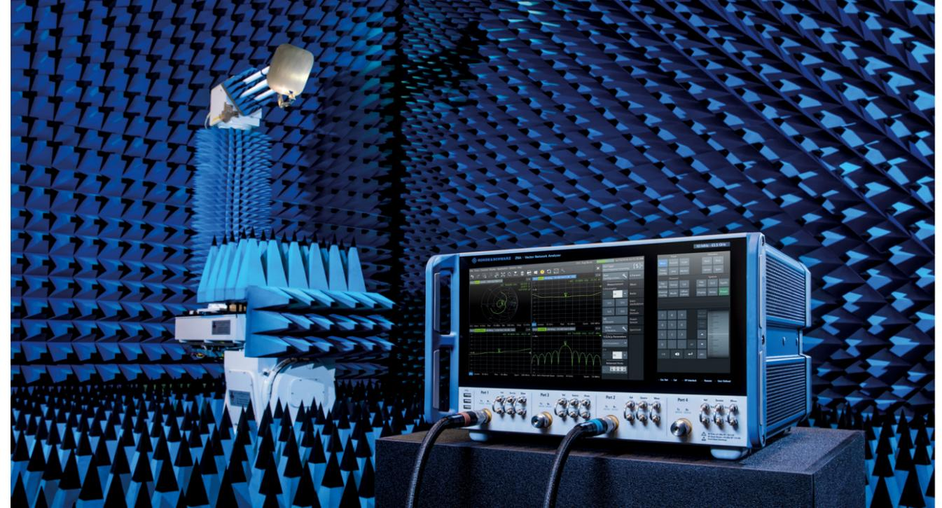
The R&S®ZNA forms the powerful core in antenna test systems.
