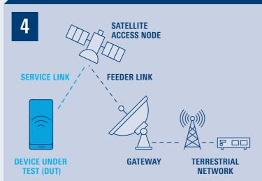
The UE is tested in an emulated terrestrial/ non-terrestrial 5G network (NTN). The solution offers full-channel emulation of NTN multiorbital (LEO, MEO, GEO/GSO) and multiband (S-, L-, Ku-, Ka-band) scenarios.
