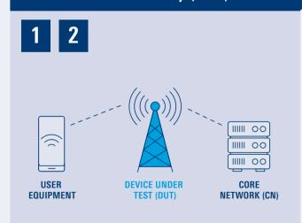
The setup offers comprehensive test coverage including network energy efficiency (NEE) of the radio access network (RAN / O-RAN) in compliance with the 3GPP conformance standards specified in TS 38.141-1/2 Chapter 6 and 7.
