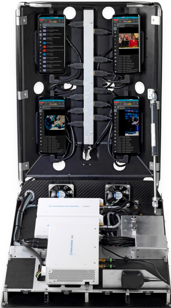
View of inside with QualiPoc, R&S®NCM4 compact integrated PC and R&S®TSME6 ultracompact drive test scanner
