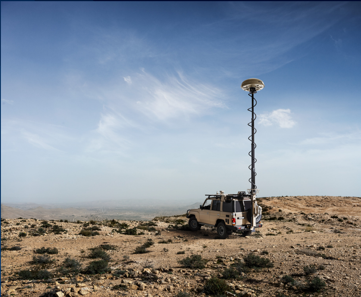
Mobile monitoring station (MMS)/mobile COMINT platform.
