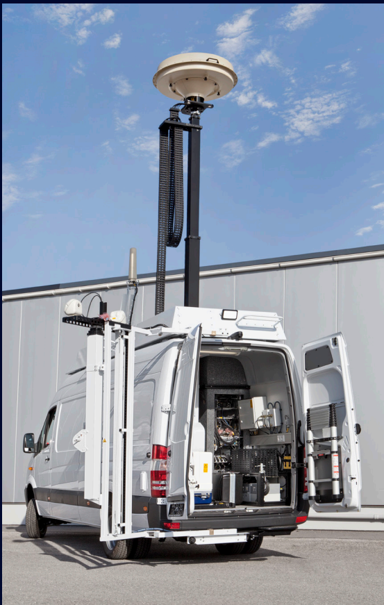
R&S®ESMW installed in a mobile monitoring station
