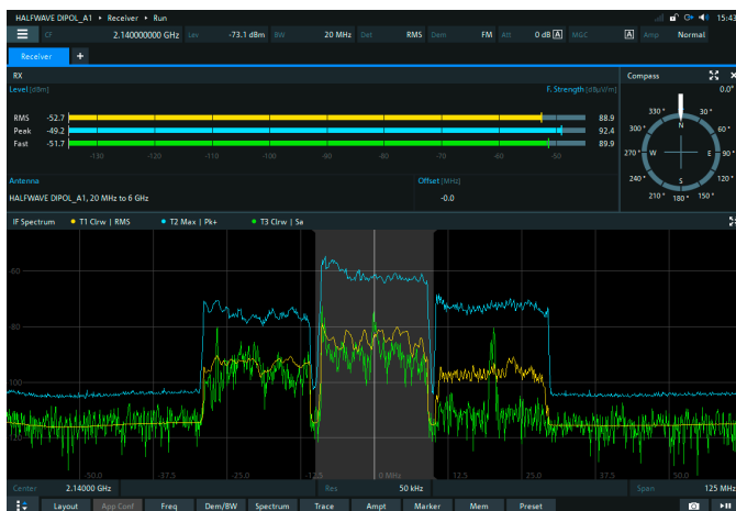
The results of up to three level detectors along with their field strength measurements can be displayed simultaneously
