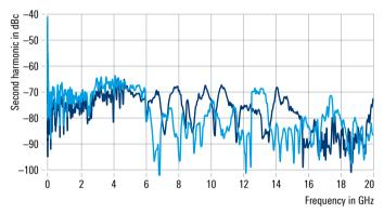
Measured at 18 dBm, with the ultra high output power option installed (R&S<sup>®</sup>SMAB-K33 + R&S<sup>®</sup>SMAB-B34)
