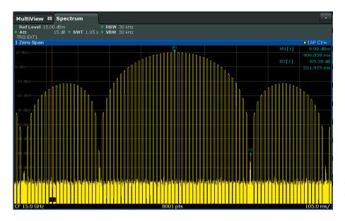
Pulse and amplitude-modulated signal generated with the R&S $^{S}$ SMA100B. The sin(x)/x modulation signal is fed at the external analog modulation input and used to produce a signal with 70 dB (meas.) modulation depth
