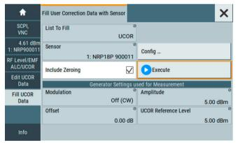
After the user correction table has been activated, the R&S<sup>®</sup>SMA100B adapts its output power to compensate for the frequency response of the RF cable.
