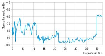
Measured at 10 dBm with the high output power option installed (R&S®SMAB-B39)
