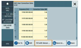
The R&S®NRP18P power sensor automatically measures and stores the frequency response of the RF cable.
