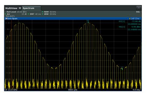
Exponential amplitude modulation with the R&S<sup>®</sup>SMA100B using the internal LF generator to deliver a sinusoidal modulation signal in order to produce a signal with 72 dB (meas.) modulation depth
