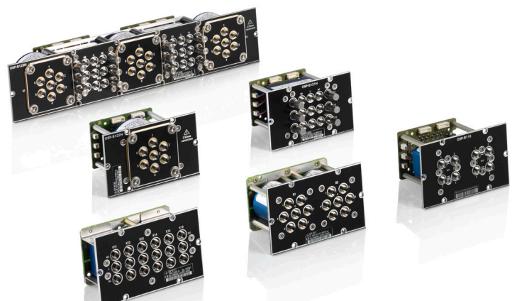
Modules with terminated and non-terminated relays from DC to 40 GHz.
