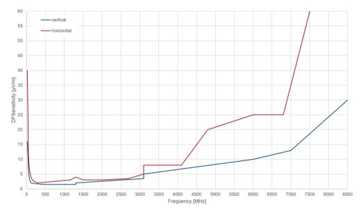
Fig. 1: DF sensitivity <sup>5</sup> (low-noise mode, 5° RMS, 5 s, 1.33 kHz (typ.))
