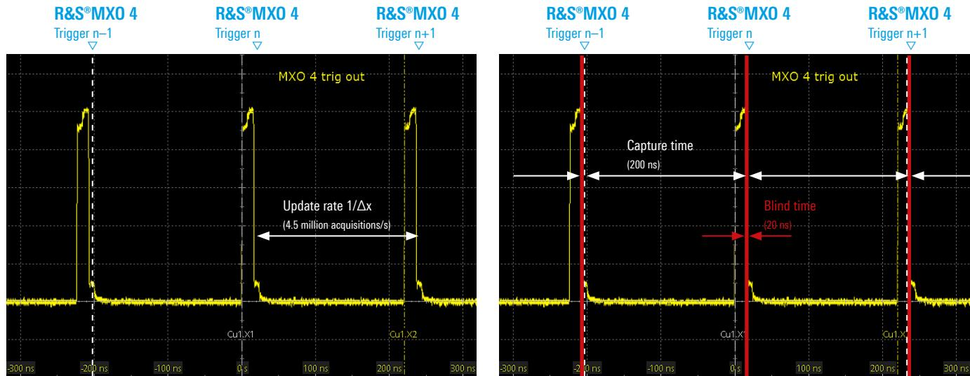
This example represents an ideal update rate measurement where the trigger out pulses are equally spaced. In reality, trigger out pulses will not always occur at regular intervals, as described later in this paper.
