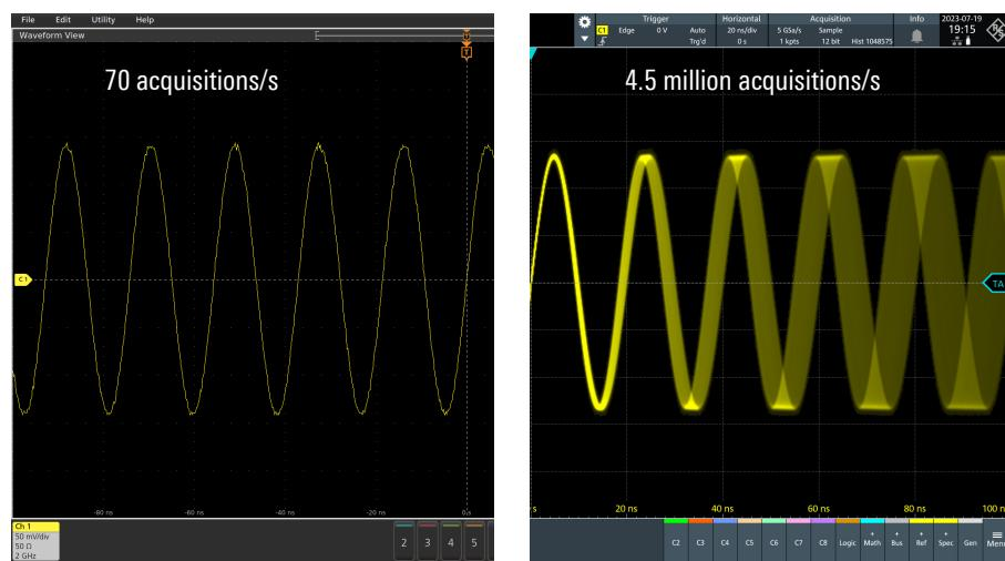
**Fig. 14: Impact of fast update rate on an oscilloscope's ability to accurately show spectral content**
