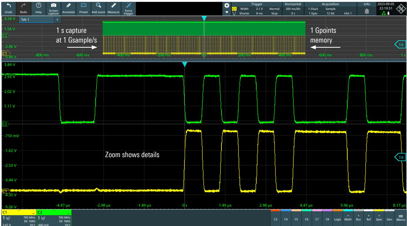
Many users want to capture a specific amount of time or as much time as they can. For a given sample rate, having more memory allows the user to capture longer periods of time. This benefit is obvious and appreciated. Additional memory depth allows the user to retain a needed sample rate or even a faster-than-needed sample rate. This provides some degree of confidence while also ensuring greater flexibility when acquiring a combination of slow and fast signals.
