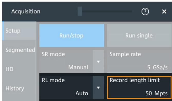
Users must manually change the oscilloscope settings to allow the instrument to use more than the artificial default limit. To make this change, users might need to enter a manual acquisition setting dialog where they can control at least the sample rate. Some oscilloscopes do not allow the user to independently control the sample rate, or the oscilloscope may not allow the user to independently control the timebase, sample rate and memory depth.
