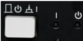
Figure 6-4: Standby switch and LEDs
