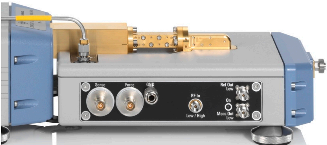
Figure 6-5: Connection between frequency converter and diplexer (var. 18)
