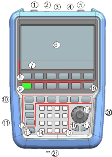
Figure 6-1: Front panel of R&S Spectrum Rider
