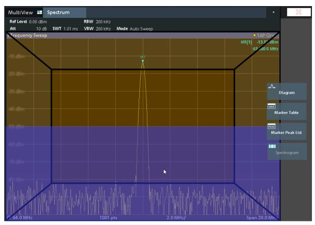
Figure 7-3: Adding a Spectrogram to the display
