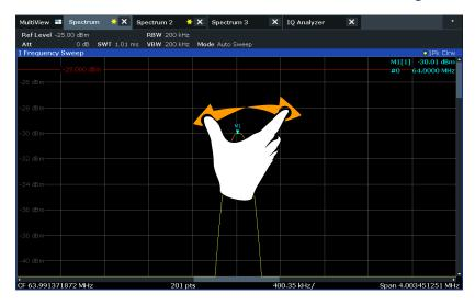
The area around the marker is enlarged in the result display.
