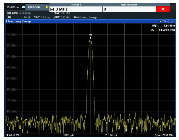
6. Now you can move the marker by tapping and dragging it to a different position. The current position is indicated by a dotted blue line. Notice how the position and value change in the marker area of the diagram.
