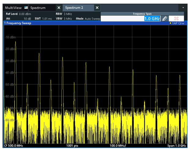
Figure 7-6: Frequency spectrum of the calibration signal with a larger span
