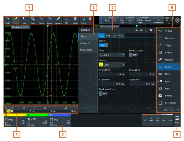
Figure 6-6: Control elements on the touchscreen
