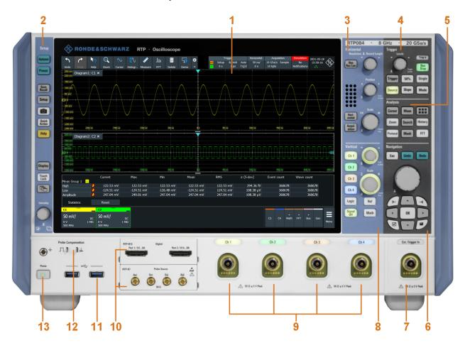
Figure 5-1: Front panel of R&S RTP
