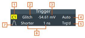
Figure 6-2: Trigger label on the toolbar
