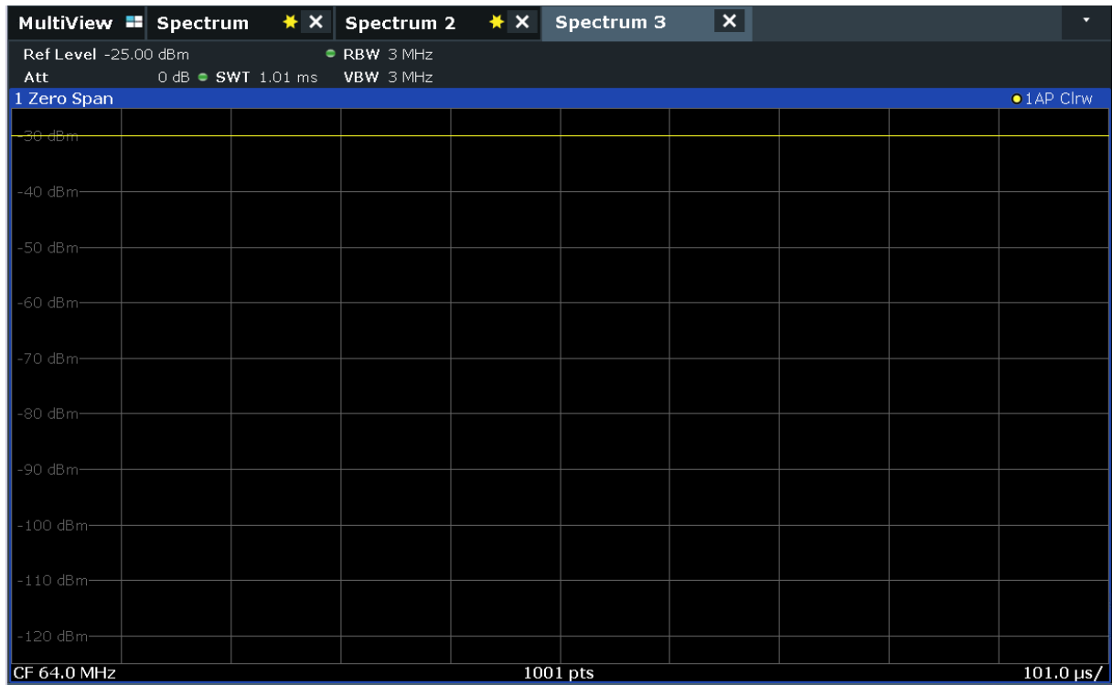
Figure 6-7: Time domain display of the calibration signal
