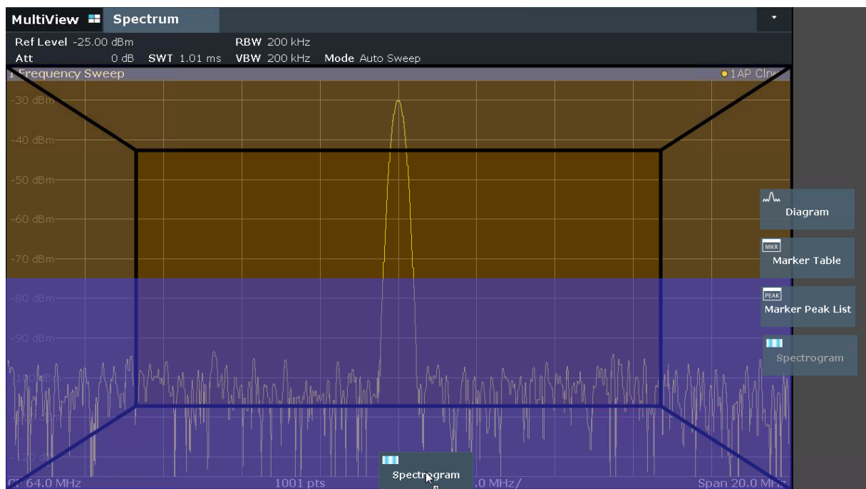
Figure 6-3: Adding a Spectrogram to the display
