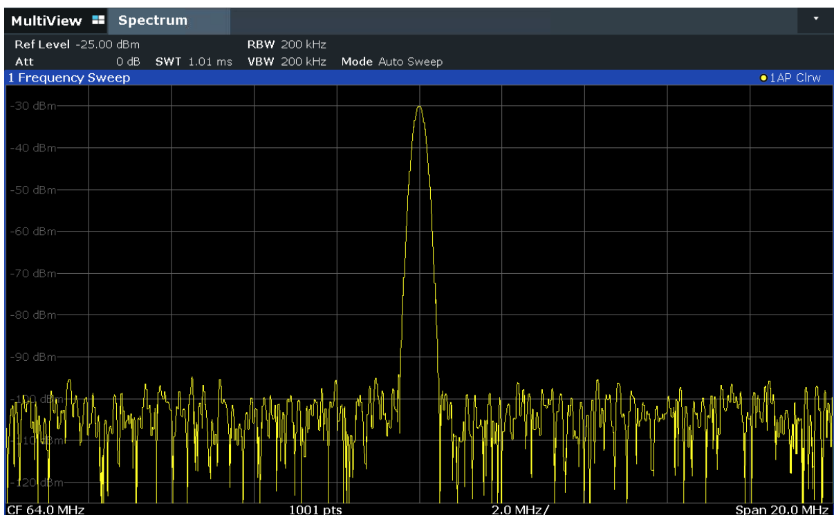
Figure 6-2: Calibration signal with optimized display settings
