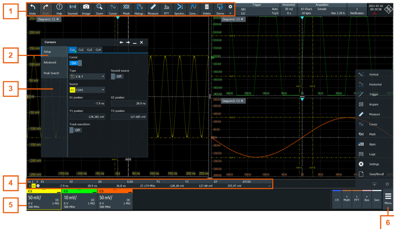
Figure 6-6: Control elements on the touchscreen
