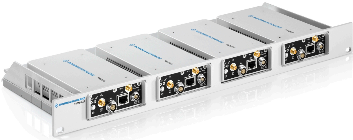
Figure 3-4: Rackmounting of 4 R&S TSME6s (reverse orientation of R&S TSME6s)
