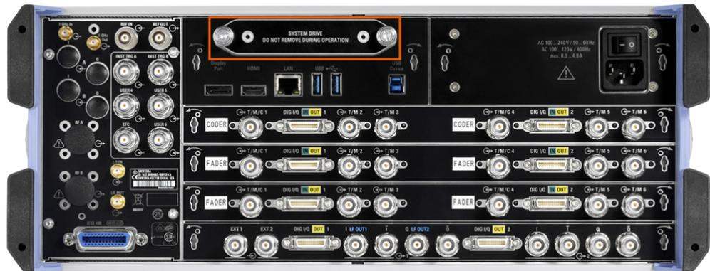
Figure 5-1: Location of the hard disk drive / solid-state drive
