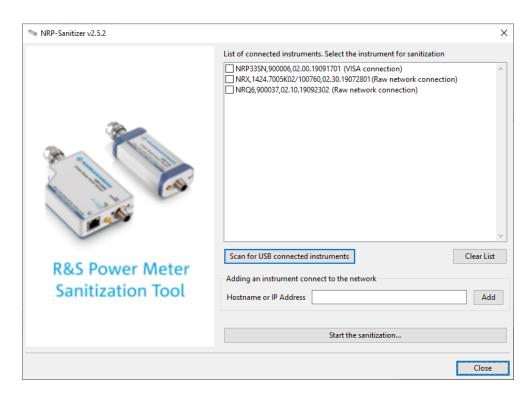
The application lists all supported instruments connected to the USB interfaces.
