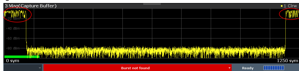
Figure 10-2: Example for incomplete burst capture
