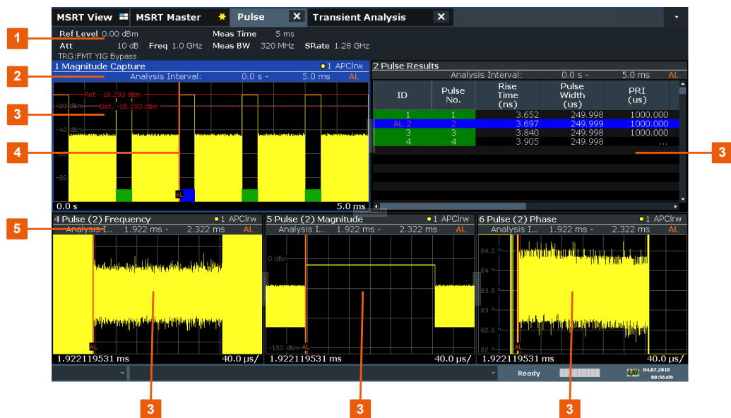
Figure 2-6: Screen elements in MSRT secondary application channels
