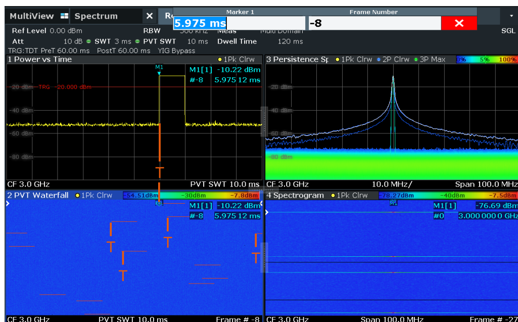
Figure 6-11: Triggered measurements in Stop on trigger mode
