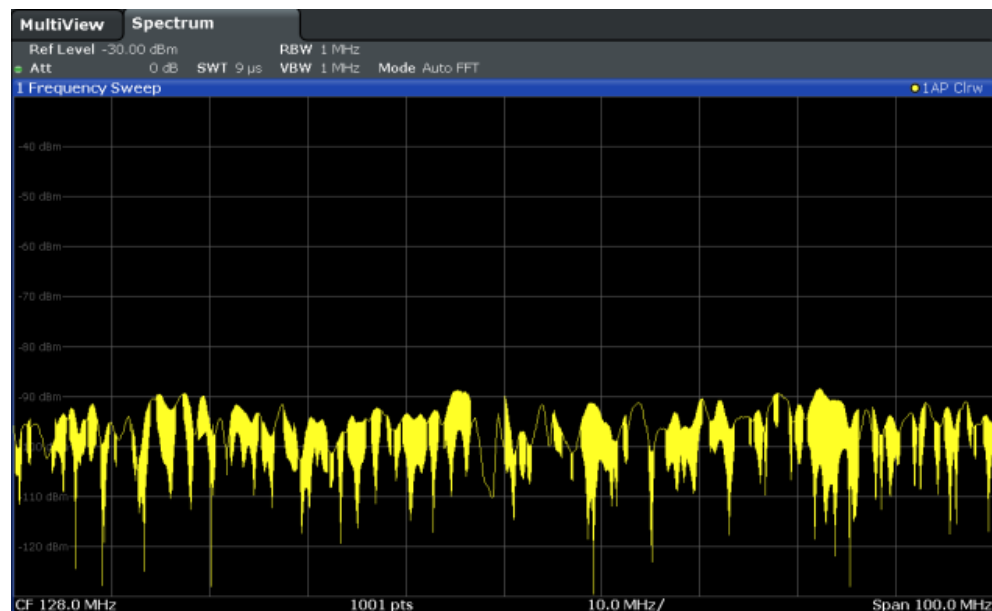
Figure 5-1: Sine wave signal with low S/N ratio
