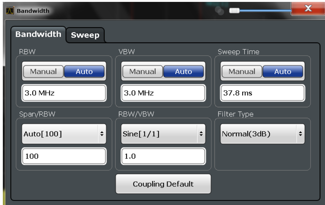
Figure 6-14: Bandwidth dialog box for RF measurements
