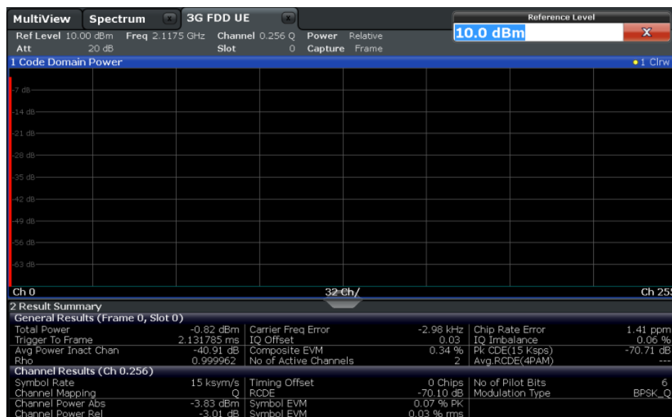
Figure 10-3: Measurement Example 3: Measuring the Relative Code Domain Power
