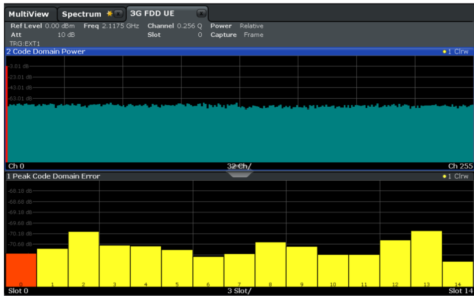
Figure 10-8: Measurement Example 6: Determining the Peak Code Domain Error
