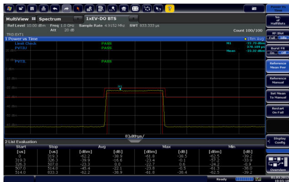
Figure 3-21: Power vs Time measurement results in the 1xEV-DO BTS application
