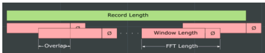
Figure 10-2: FFT parameters for averaged FFT calculation
