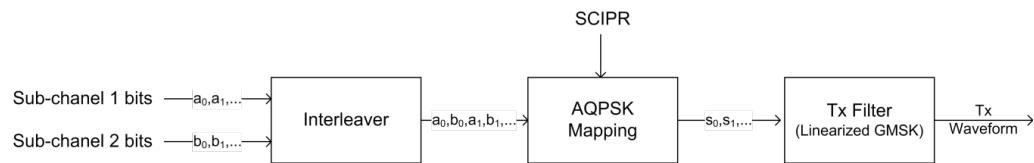
Figure 5-3: AQPSK modulation scheme for GSM systems
