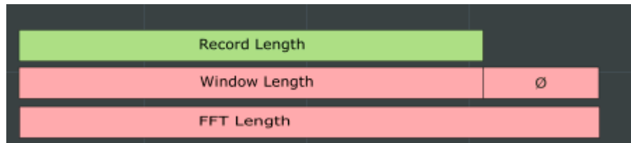
Figure 4-4: FFT parameters for single FFT calculation
