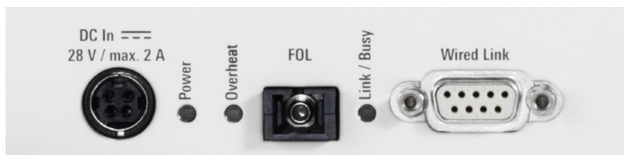
Figure 4-148: Connectors and LEDs on the rear panel of the R&S OSP-B200S2
