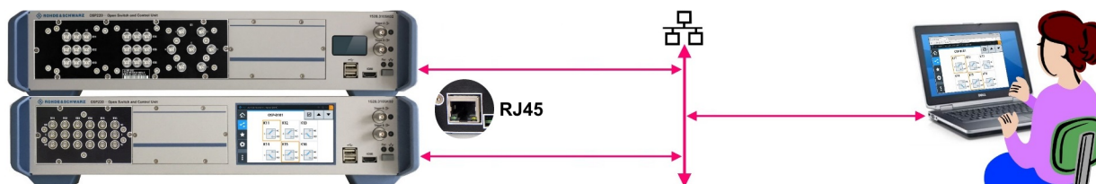
Figure 3-14: Manual remote operation via "WebGUI" and LAN
