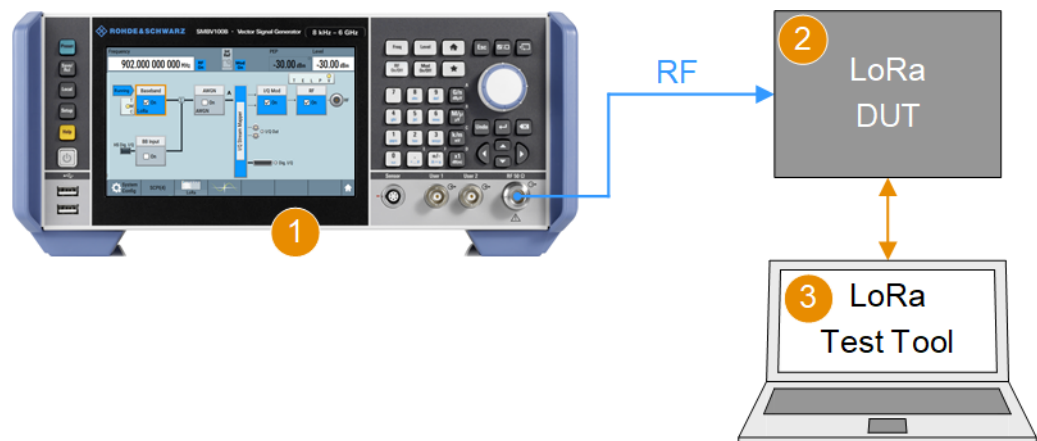
Figure 5-1: Test setup for Rx sensitivity test
