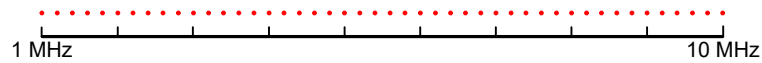
Figure 3-15: Linear x-axis scaling: the distance between the sweep points is equal, e.g. 200 kHz
