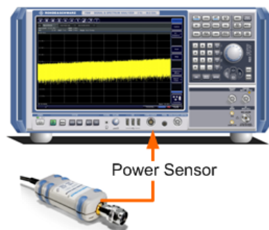
Figure 3-2: Connecting a power sensor using the POWER SENSOR interface
