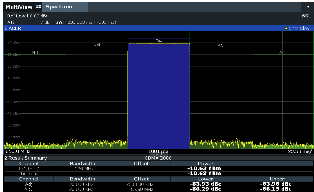
Figure 2-21: Measuring the channel power and adjacent channel power ratio for CDMA2000 signals with zero span (Fast ACLR)
