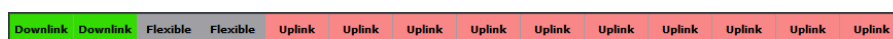
Figure 4-6: Preview of symbol usage for slot format 38 as defined in 3GPP 38.211, table 4.3.2-3
