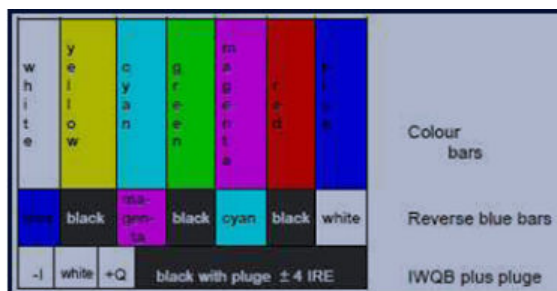
Figure 2-10: Detail description on SMPTEBARS
