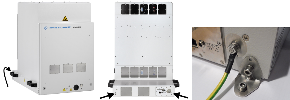
Figure 6-3: Positions of the mounting brackets for fixing the chamber to its support
