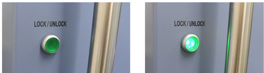
Figure 7-1: Light in the door's [LOCK / UNLOCK] button
