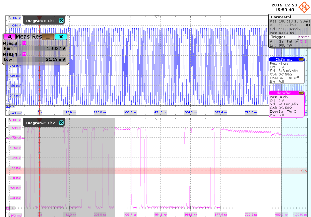
Figure 4-4: HS200 CMD Push Pull input level voltage
