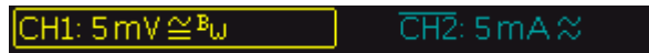
Figure 5-1: Channel labels: Channel 1 is selected, is DC coupled and bandwidth limited. Channel 2 is AC couples and inverted.
